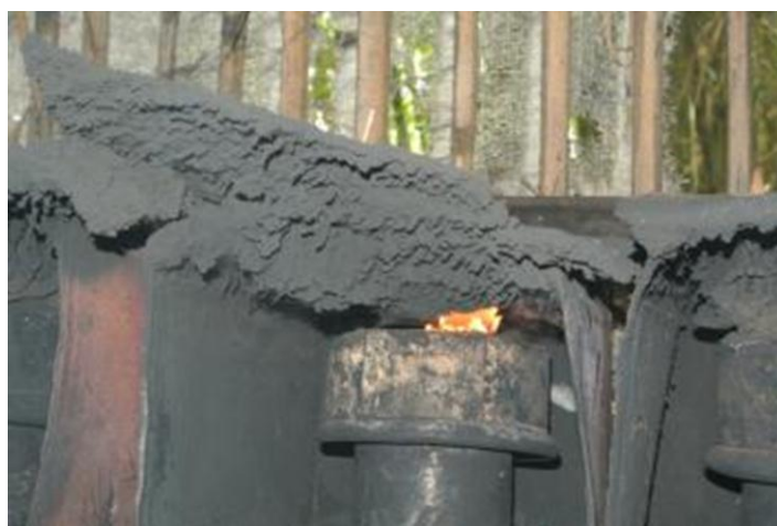
Figure 3.1: A form of flame carbon prepared by burning kerosene oils. The soot produced in the cracker container gradually became thick and swept out by means of a feather brush.
